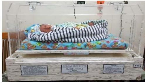
Gambar 2. Inkubator bayi portable tanpa baterai emergensi [5]
