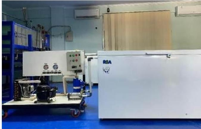
**Gambar 1.** Trainer sistem *Air cooled chiller*
