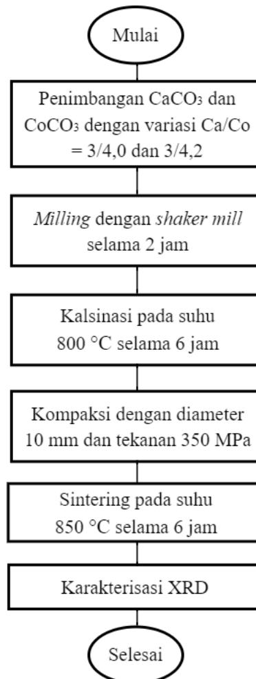
Gambar 2. Diagram alir percobaan sintesis polikristal \text{Ca}_3\text{Co}_4\text{O}_9 .
